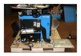
**Step 5:** Install the pneumatic control switch into the wheel lift cover as shown.
