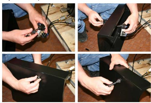
**Step 6:** Install the wheel lift cover over the front of the wheel lift and attach it to the tire changer chassis with the provided hardware. On TC733 models, the holes will be predrilled from the factory. It may be necessary to thread these holes with a 6mm x 1.0 tap. On all other Atlas models, you must drill and tap these holes using the cover as a template.
