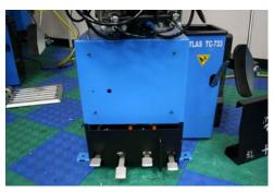
**Step 3:** On TC733 models, the mounting holes for the wheel lift are pre-drilled (arrows). It may be necessary to thread some of these holes using a 6mm x 1.0 tap.
