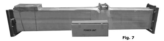
2. Move the lift aside with a forklift or hoist, and open the outer packing carefully , take off the parts from upper and inside the column, take out the parts box, check the parts according to the shipment parts list (See Fig. 8).
