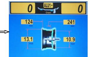
• Move the AD gauge to the position "2" as shown in the figure 19. Two seconds later, the dimensions AE and DE are set automatically, and a beep sound is heard in the meantime. The set dimensions are shown on the screen after releasing the gauge.
