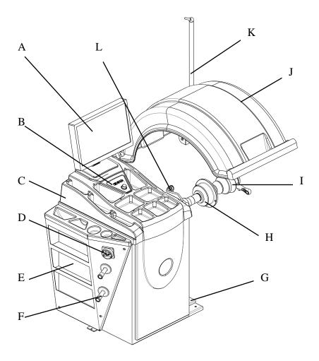
A: LCD monitor B: Control panel C: Wheel weight tray D: Main switch E: Tool shelf F Cone holder G: Foot brake H: Balancing shaft I: Quick nut and cones J: Wheel guard L: B gauge K: A/D gauge
