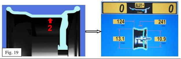
The positions "1" and "2" are determined by the operator according to the rim profiles. The distance between two positions must be more than 2.5 inch. Failure to do so, the measurements cannot be correct.
