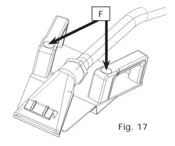
fig.17), then press the buttons (F) all the way down: a strong jet will be released through the nozzles in the slides and this will help the bead seal. Make sure to hold the blasting handles firmly during this operation.
