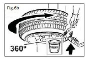
To break the lower bead of the tire, do as follows:
