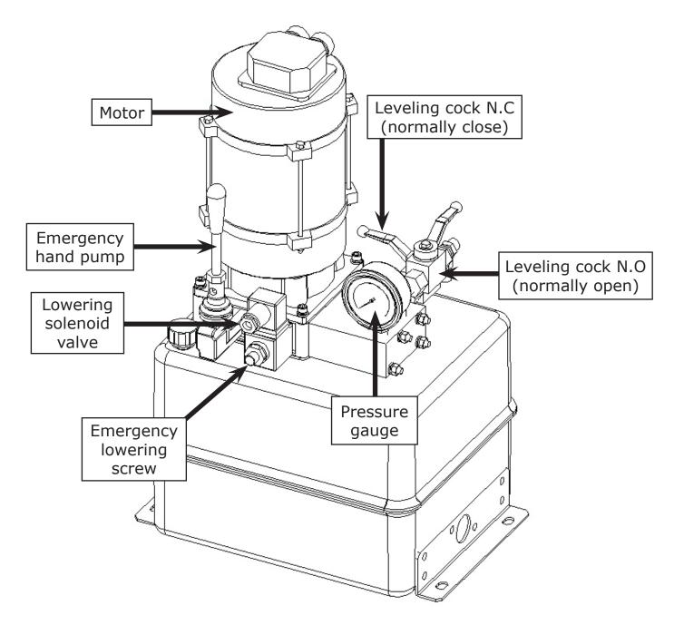
Figure 3 – Hydraulic Power Unit
