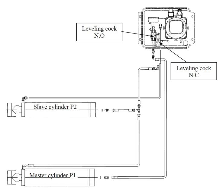
Figure 14 – Hydraulic Connections
