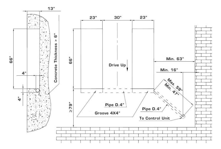
Figure 13 - Pit Foundation Plan
