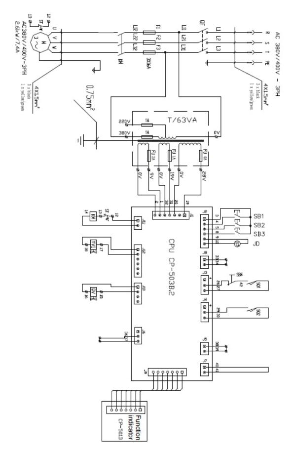
Figure 5a – Electric Diagram (380V/400V - 3PH)
