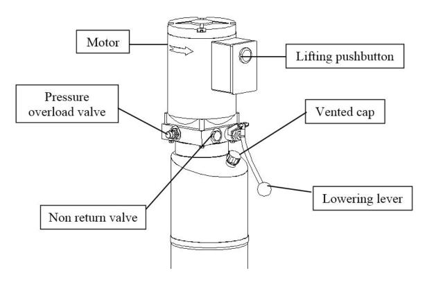
Figure 4 – Hydraulic Power Unit
