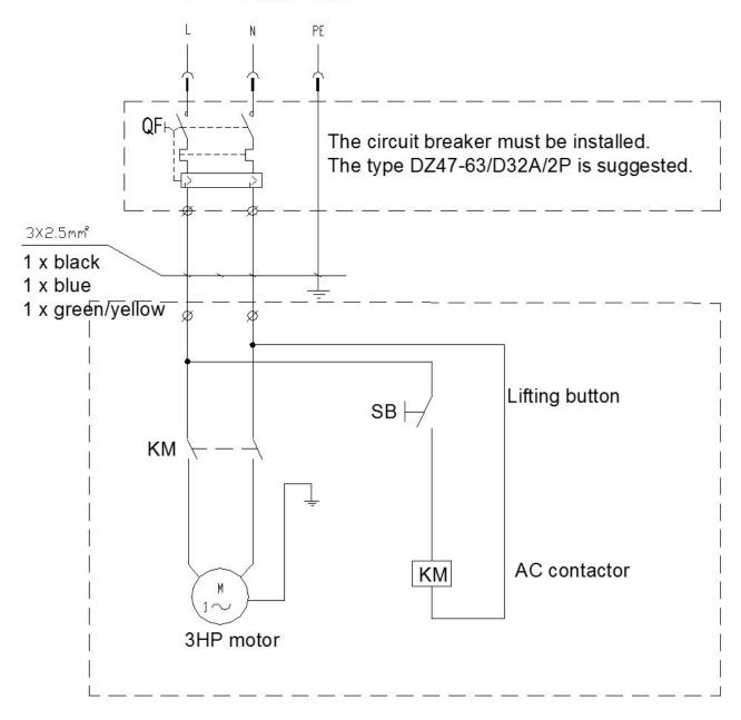
Figure 6 – Electrical Diagram (220V/50Hz/60Hz/1Ph)
