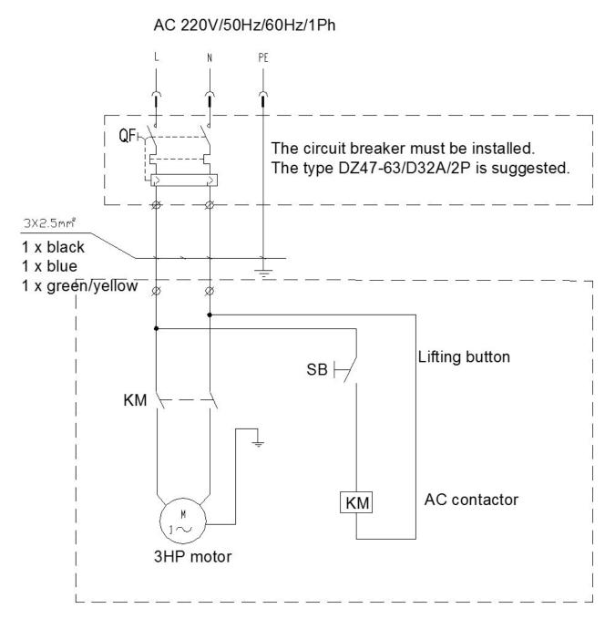
Figure 6 – Electrical Diagram (220V/50Hz/60Hz/1Ph)
