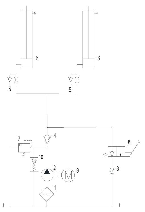
Figure 5 - Hydraulic Plan
