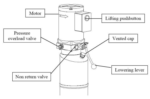
Figure 4 – Hydraulic Power Unit
