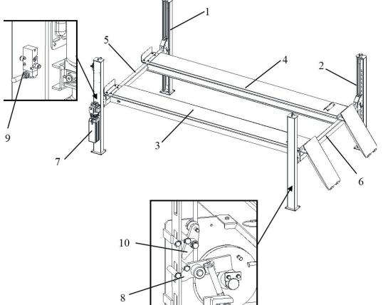
The automatic mechanical back-up safety (8) holds on the lift in the elevated position, can be released by pushing the lever of the control valve (9). The slack cable safety (10) can hold on the lift in event of cable slackening and/or failure.
