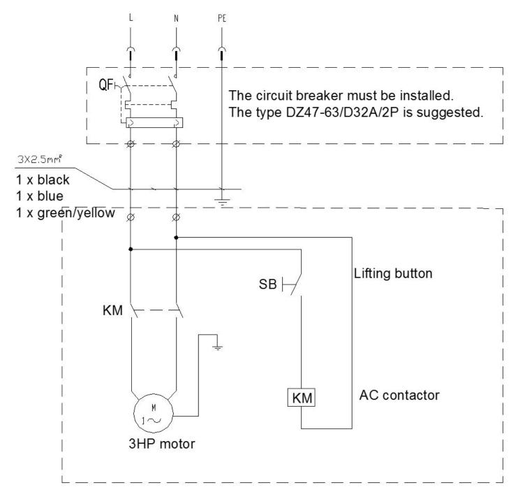
Figure 6a – Electrical Diagram (220V/230V/50Hz/60Hz/1Ph)
