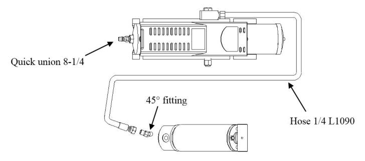
Figure 24 – Hydraulic Line Connection Of Jacking Beam
