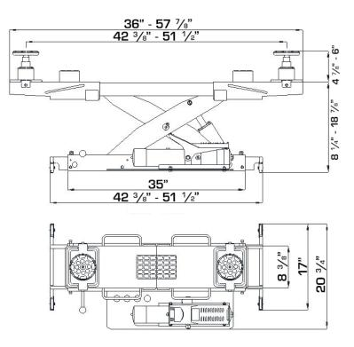
Figure 22 – Jacking Beam Layout
