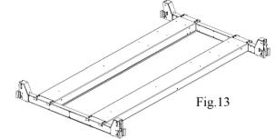
accessories are installed in the runways before installation. Make sure that the plastic slide blocks are in position.
