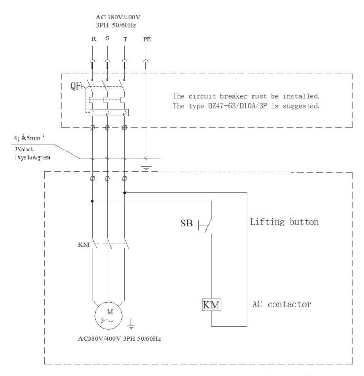
Figure 6b - Electrical Diagram (380V/400V/50Hz/60Hz/3Ph)
