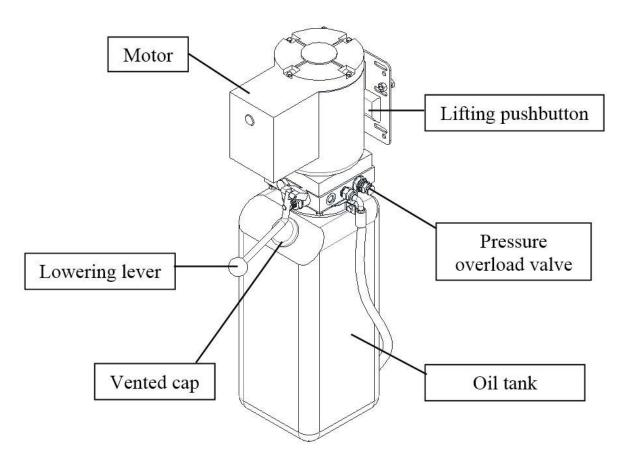
Figure 4 – Hydraulic Power Unit
