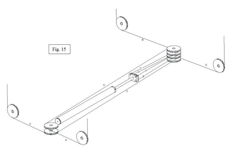
Figure 15 – Cable Routing Diagram
