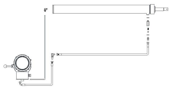
Figure 17 – Hydraulic Line Connection
