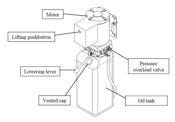
Figure 4 – Hydraulic Power Unit
