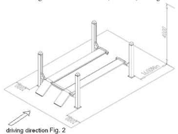
2. FLOOR REQUIREMNETS: The lift should be installed on a 3000 PSI concrete with little gradients. Thickness of concrete ≥ 6 inch (150 mm). The leveling of whole area ≤ 3/8 inch (10 mm). Or, every column shall be located on a concrete block with size at least 24\*24 inch (600\*600 mm), thickness ≥8 inch (200mm)
